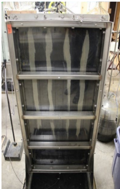
Figure 3 Image of a flow-through tank in operation. Dark areas show PlumeStop in the more conductive area and start to diffuse into the lower k zones (lighter color bands).
