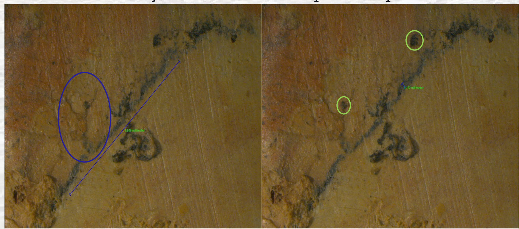
The picture shows petite seams within a very fine-grained clay. If one looks closely branching can be seen. Branching is circled in blue. Note also that PAC seams are also directed toward the viewer. A couple of examples are circled in green.
