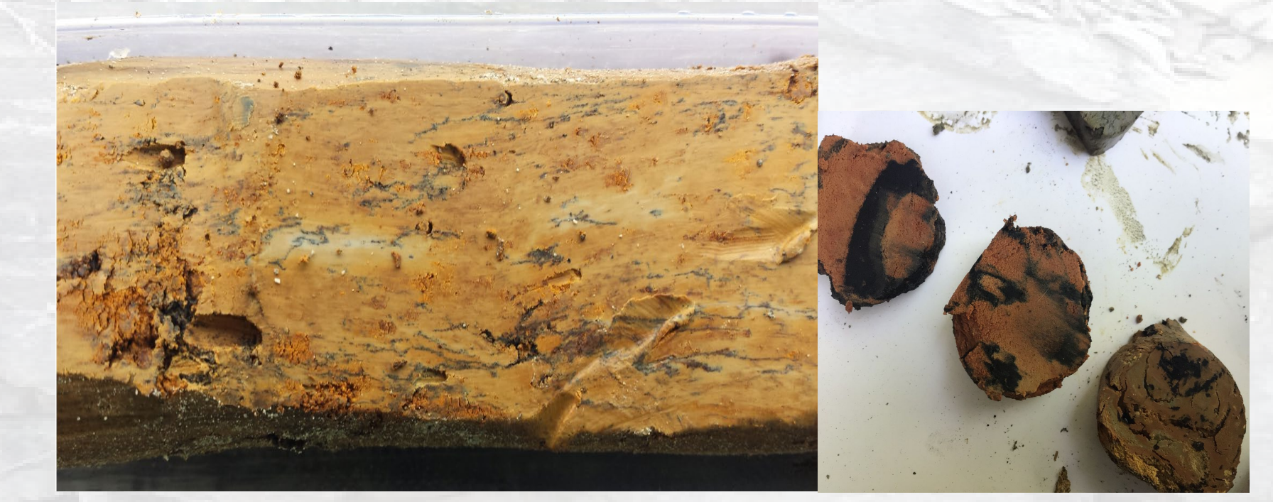
The BOS 200® is injected using sufficient pressure to facilitate localized soil lifting and propagation from the injection tip. Injection pressures typically vary from 200 to 600 psig as measured at the discharge end of the injection pump. In fine-grained sediments (clays and silts) there is typically a soil lifting pressure that is momentarily sustained after which the pressure drops off to a propagation pressure. In coarse-grained sediments (sands and fine gravels), a steady progression pressure is typically displayed as the lithology near the injection tip is fluidized and turbulent flow is created.
