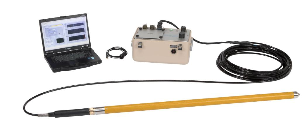
The DP NMR tools are operated by an NMR Surface station and logging cable which are connected to the NMR Tool. The control unit is powered by a 24VDC battery pack.
