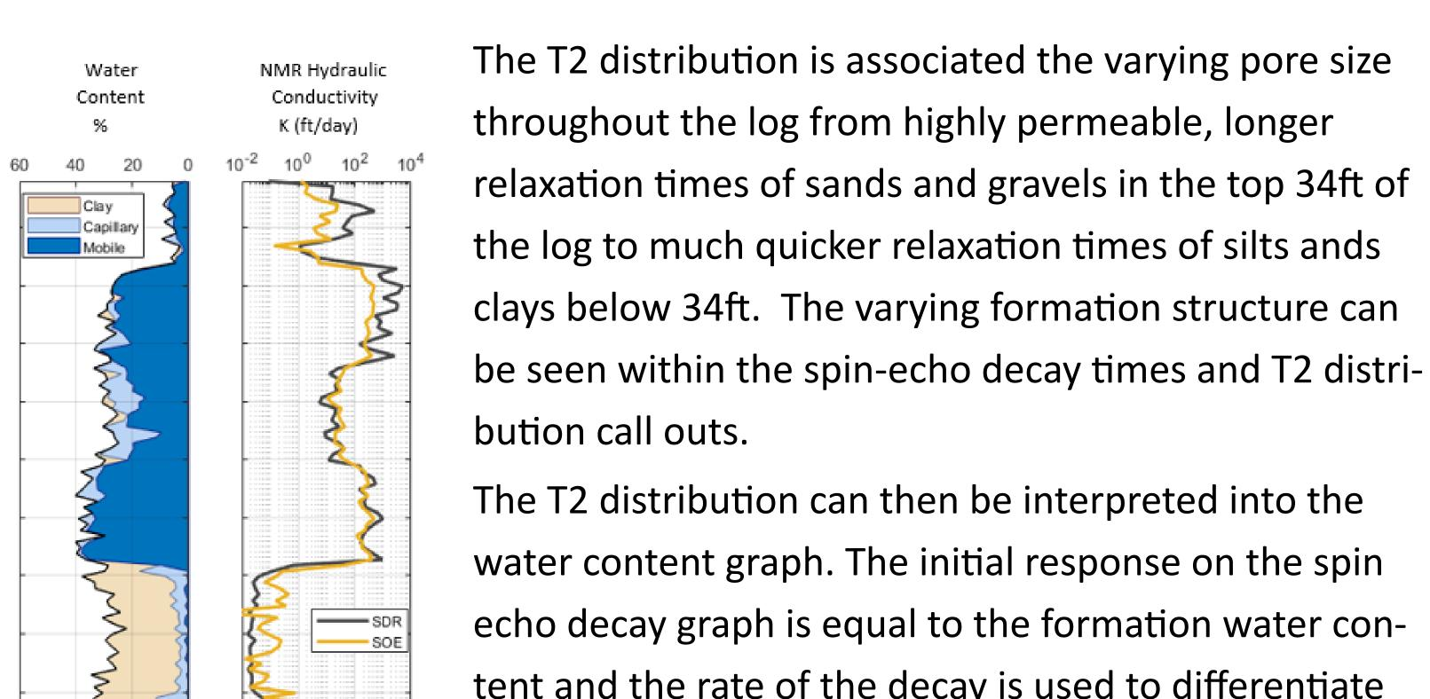
The T2 distribution can then be interpreted into the water content graph. The initial response on the spin echo decay graph is equal to the formation water content and the rate of the decay is used to differentiate between "mobile" water in high permeable formations and "bound" water in silts and clays. The processing software also generates two models of hydraulic conductivity (k) including Schlumberger-Doll research and the sum-of-echoes equations.
