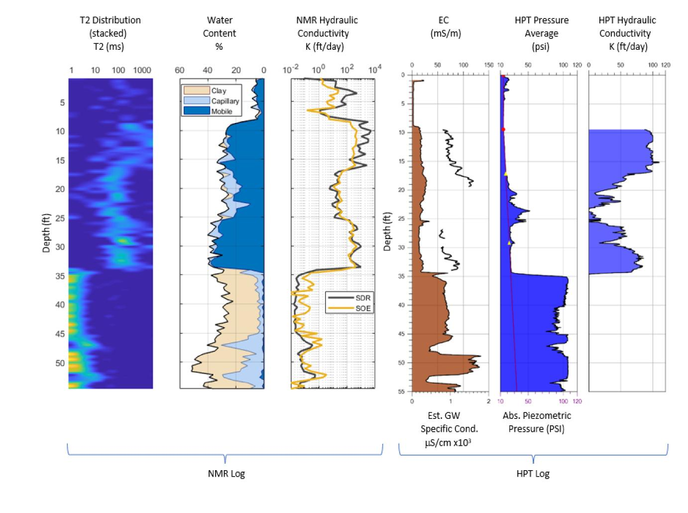
This NMR log was collocated with an HPT log which confirm the static water level at approximately 9ft, a highly permeable aquifer between 8-34ft as well as some silty material between 20-25ft and a couple slightly more permeable zones between 45-55ft. The HPT K estimation reaches its model limits of ~75ft/day in the top 7ft of the aquifer and between 30-35ft. The NMR models can effectively estimate hydraulic conductivity an order of magnitude above and below the HPT estimations.
